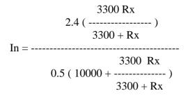
Where Rx is the value to be used for both resistors.
